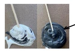
3rd mix the 2-part epoxy until you get the desired color instructed with this epoxy mix that it's been fully mixed, and ready to use.
