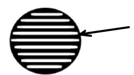
Vents are on the underside of the units, which allows the fans to properly vent and cool down the system from below, which look like this image. 2 Burners will have 1 vent, 3 and 4 Burners will have 2 vents and 5 Burner will have 3 vents that must not be obstructed.
